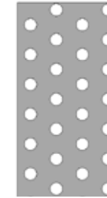
5/8" diameter staggered tubes
