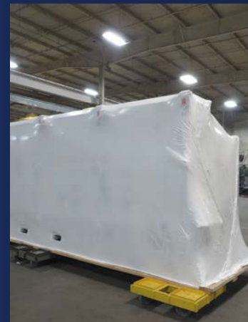
Shrink-Wrapped Equipment: Arrives at the jobsite in factory condition for installation or storage
