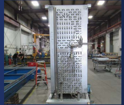
Stainless Steel Venturi Distributor: Ensures uniform refrigerant distribution and enhanced heat transfer
