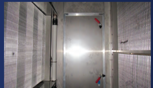
Hygienic Construction & Materials: The interior features stainless steel construction throughout, including fully seal-welded sloped drain pans that eliminate standing water and prevent microbial growth. The exterior is G235 galvanized steel for long-term corrosion resistance in washdown environments.
