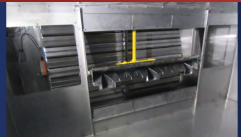
Direct-Fired Burner: 100°F-rise burner with wide turn-down. Enables full cleanup mode from sub-zero winter air to warm summer conditions.
