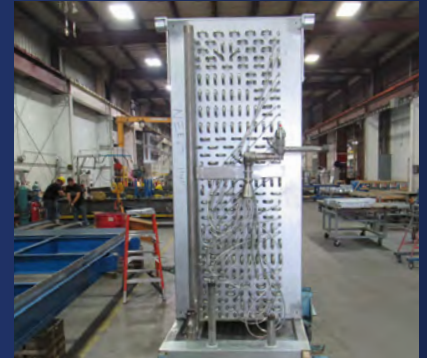
Stainless Steel Venturi Distributor: Ensures uniform refrigerant distribution and enhanced heat transfer
