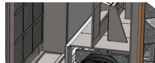
05 Fresh Air Dampers
