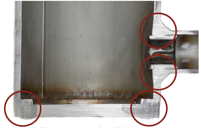
Full Penetration Header Weld Joints
