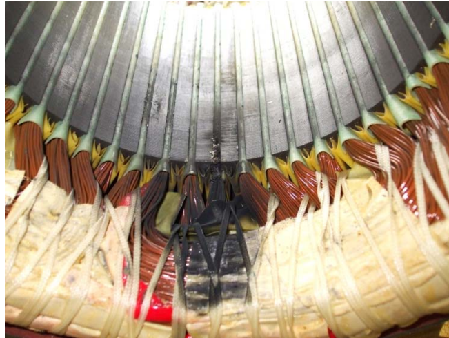
Figure 2 Motor Insulation Failure Resulting From Corona Effect
