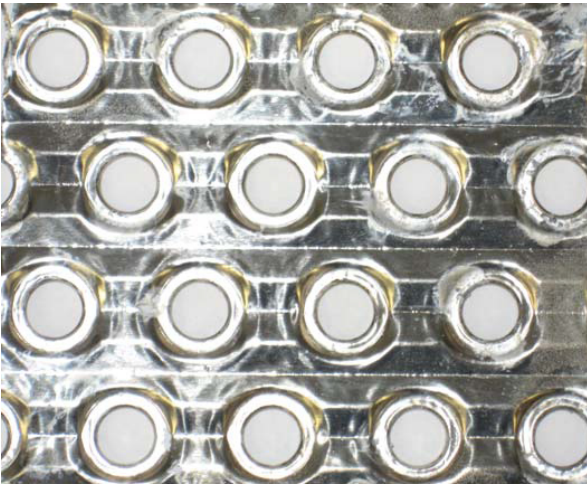
Figure 48: 5052 Aluminum after 250 hours submerged in a .16% Sunny-Sol 150 water solution
