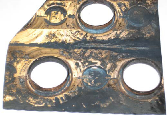
Figure 56: Copper-nickel 95/5 after 500 hours submerged in a 10% ammonium hydroxide solution
