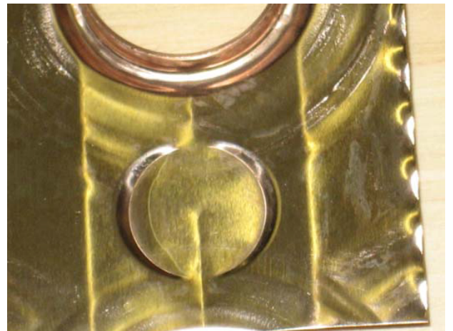
Figure 26: 95/5 Copper-nickel after 250 hours submerged in a 3.9% FRM 63-CB water solution
