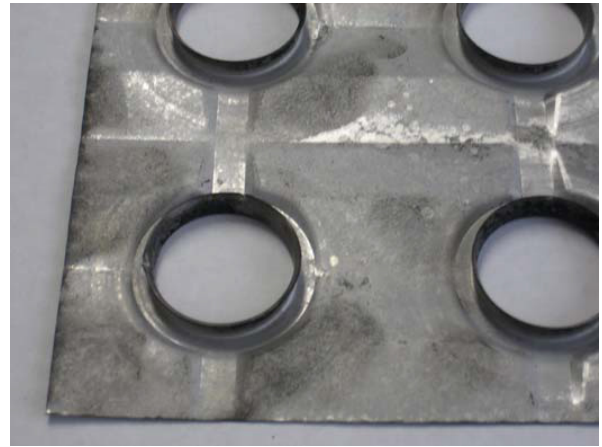
Figure 59: 1100 series aluminum after 500 hours submerged in a 10% ammonium hydroxide solution
