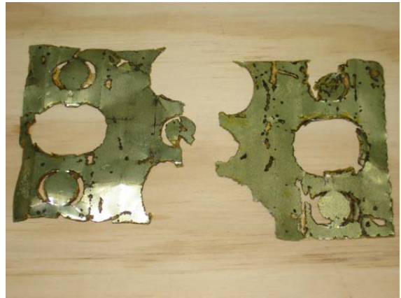
Figure 30: Aluminum polycoat after 250 hours submerged in a 3.9% FRM 63-CB water solution
