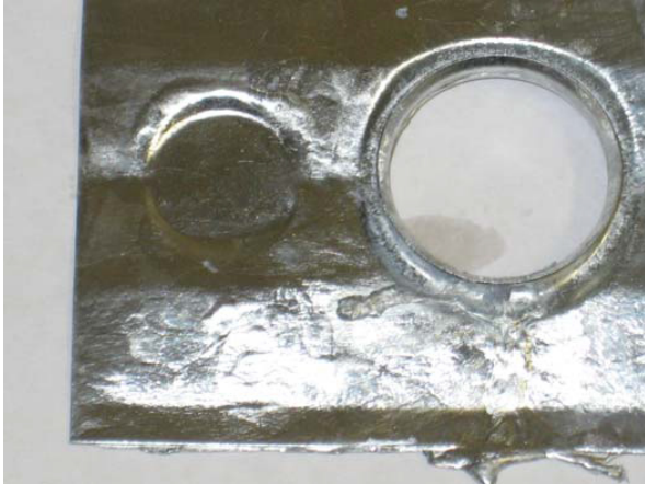
Figure 51: Hot dipped galvanized steel sample before corrosion testing
