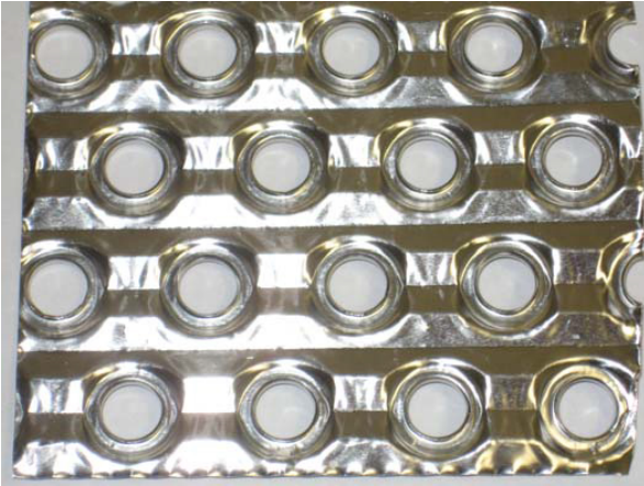
Figure 47: 5052 Aluminum sample before corrosion testing
