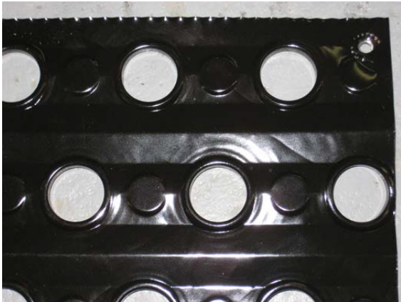
Figure 32: Aluminum Electrofin sample before corrosion testing
