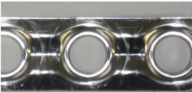
Figure 38: 304 Stainless steel after 250 hours submerged in a .16% Sunny-Sol 150 water solution
