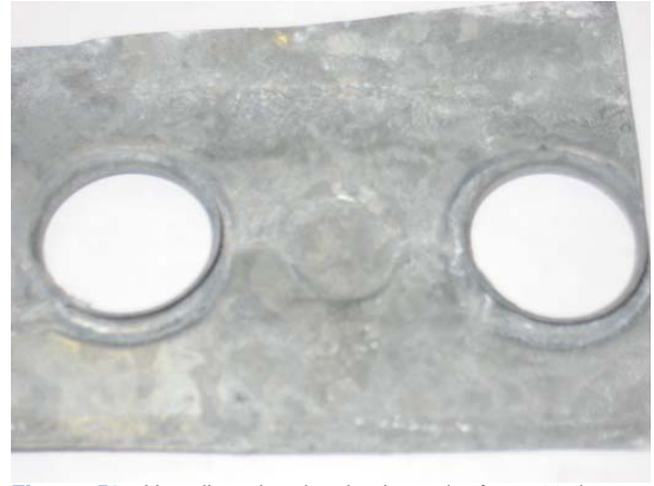
Figure 58: Hot dipped galvanized steel after 500 hours submerged in a 10% ammonium hydroxide solution
