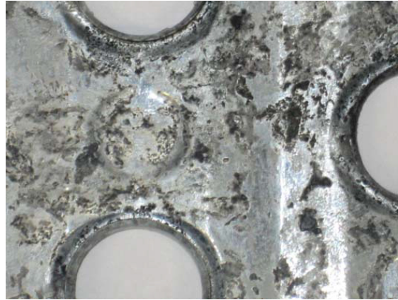
Figure 53: Hot dipped galvanized steel after 250 hours submerged in a .16% Sunny-Sol 150 water solution
