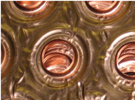
Figure 2: Copper C11000 sample before corrosion testing
