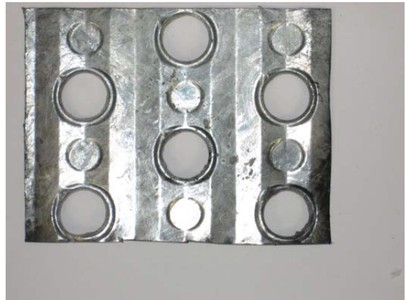
Figure 55: Hot dipped galvanized steel after 250 hours submerged in a 3.9% FRM 63-CB water solution
