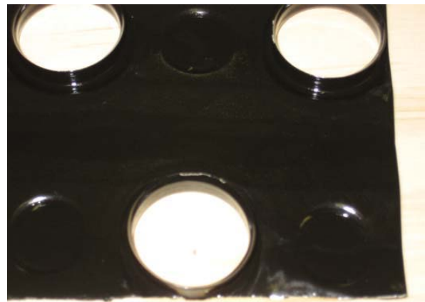
Figure 36: Aluminum Electrofin after 250 hours submerged in a 3.9% FRM 63-CB water solution
