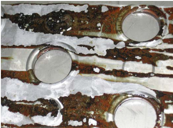
Figure 13: Carbon steel after 250 hours submerged in a .16% Sunny-Sol 150 water solution
