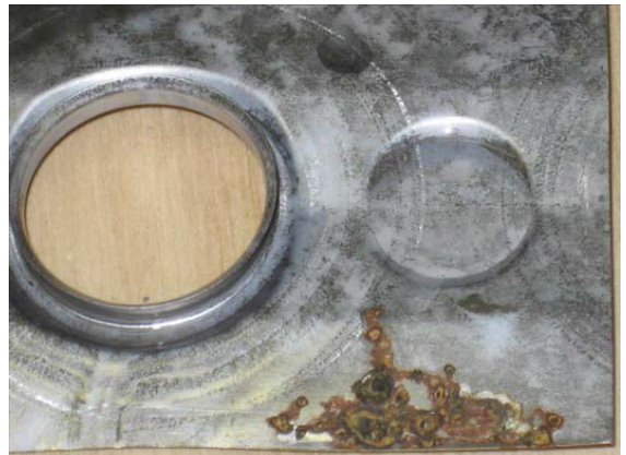
Figure 16: Carbon steel after 250 hours submerged in a 3.9% FRM 63-CB water solution
