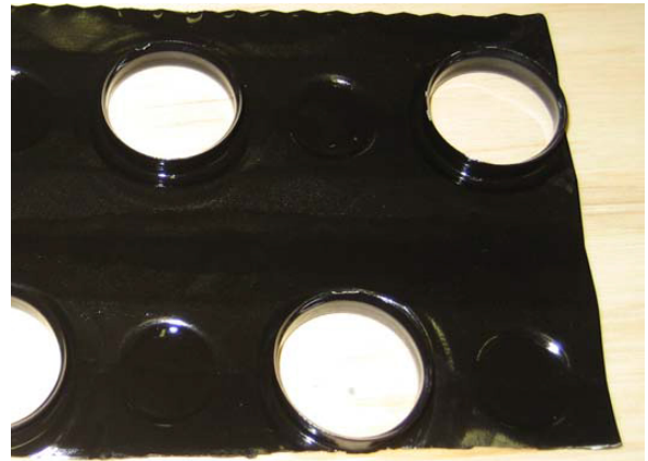
Figure 35: Aluminum Electrofin after 250 hours submerged in a 3.9% FRM 63-CB water solution
