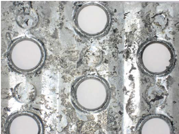
Figure 52: Hot dipped galvanized steel after 250 hours submerged in a .16% Sunny-Sol 150 water solution
