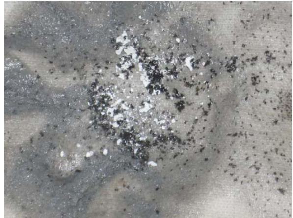
Figure 10: Aluminum 1100 after 250 hours submerged in a 3.9% FRM 63-CB water solution
