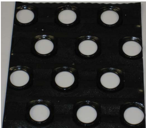
Figure 43: Black Heresite after 250 hours submerged in a .16% Sunny-Sol 150 water solution
