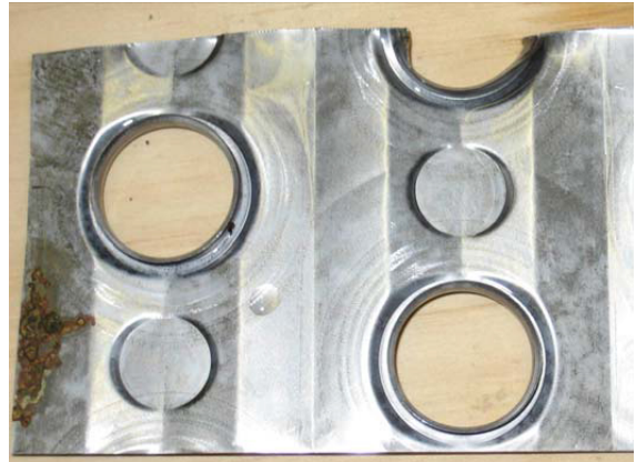
Figure 15: Carbon steel after 250 hours submerged in a 3.9% FRM 63-CB water solution
