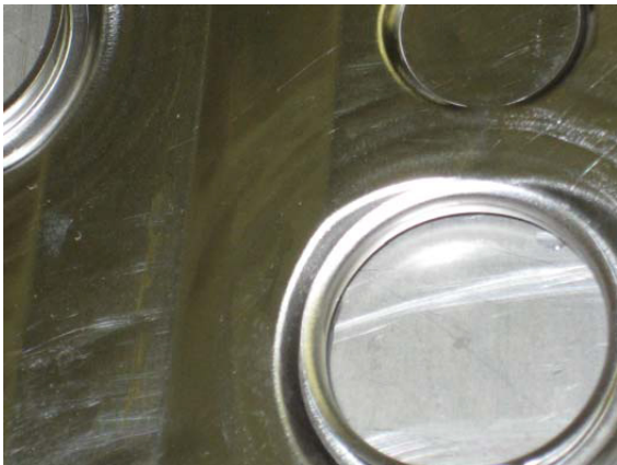
Figure 19: 316 Stainless steel after 250 hours submerged in a .16% Sunny-Sol 150 water solution
