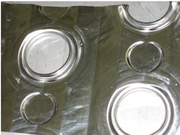
Figure 18: 316 Stainless steel after 250 hours submerged in a .16% Sunny-Sol 150 water solution
