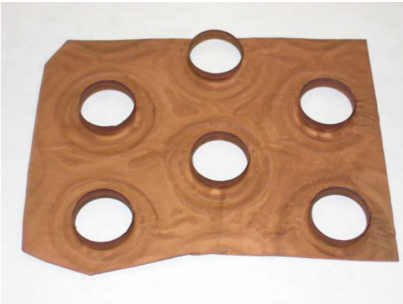
Figure 57: Copper C11000 after 500 hours submerged in a 10% ammonium hydroxide solution
