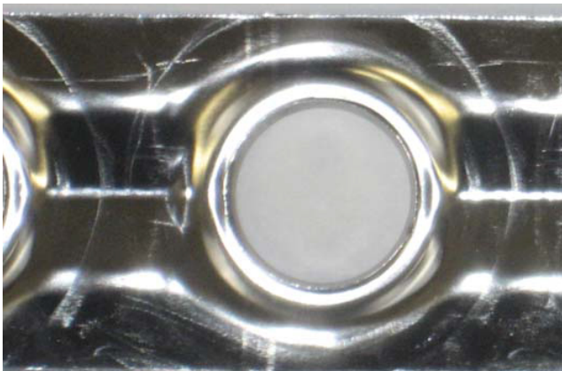
Figure 39: 304 Stainless steel after 250 hours submerged in a .16% Sunny-Sol 150 water solution
