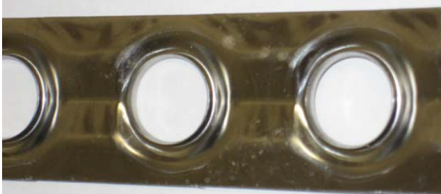
Figure 37: 304 Stainless steel sample before corrosion testing
