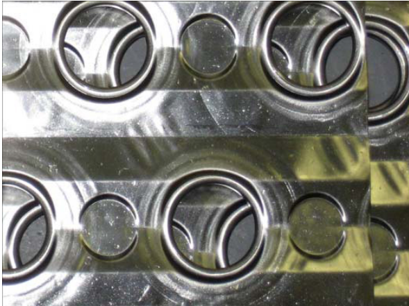
Figure 17: 316 Stainless steel sample before corrosion testing
