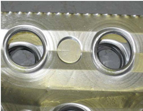
Figure 7: Aluminum 1100 sample before corrosion testing
