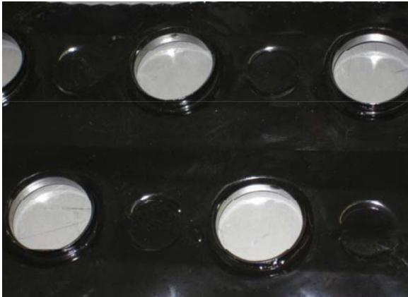
Figure 33: Aluminum Electrofin after 250 hours submerged in a .16% Sunny-Sol 150 water solution
