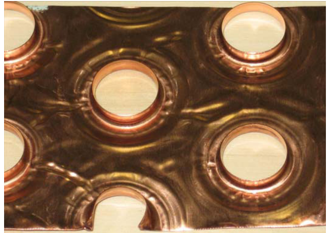
Figure 5: Copper C11000 after 250 hours submerged in a 3.9% FRM 63-CB water solution
