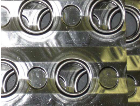
Figure 17: 316 Stainless steel sample before corrosion testing
