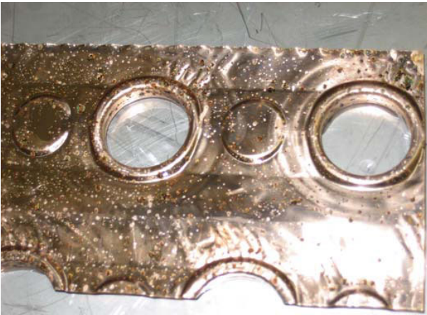
Figure 23: 95/5 Copper-nickel after 250 hours submerged in a .16% Sunny-Sol 150 water solution
