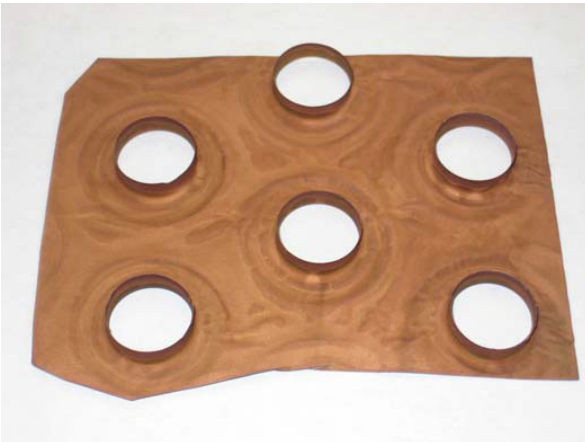
Figure 52: Copper C11000 after 500 hours submerged in a 10% ammonium hydroxide solution
