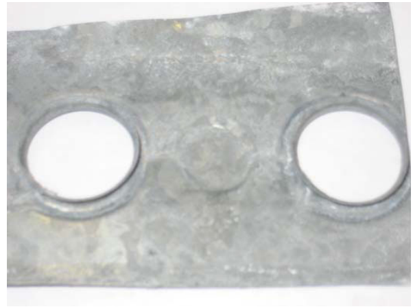
Figure 53: Hot dipped galvanized steel after 500 hours submerged in a 10% ammonium hydroxide solution
