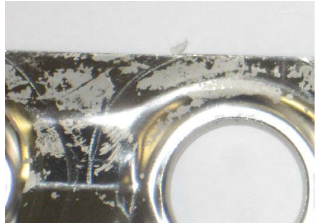
Figure 41: 304 Stainless steel after 250 hours submerged in a 3.9% FRM 63-CB water solution
