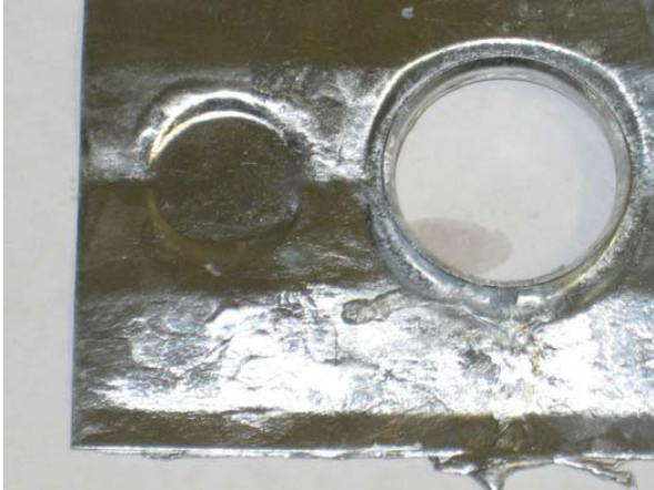
Figure 46: Hot dipped galvanized steel sample before corrosion testing
