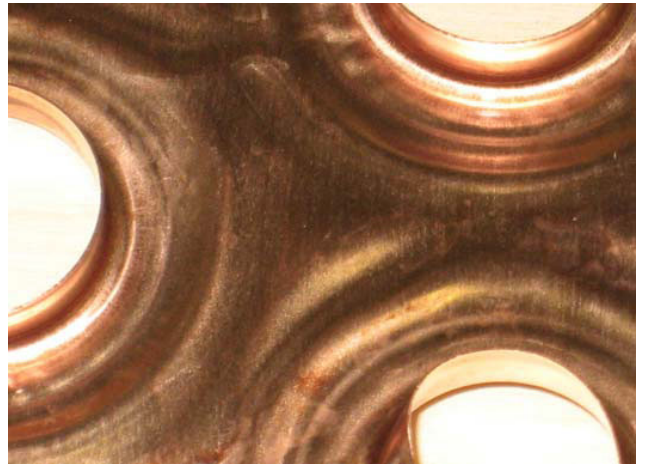
Figure 6: Copper C11000 after 250 hours submerged in a 3.9% FRM 63-CB water solution
