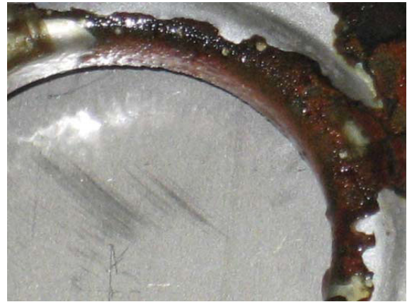
Figure 14: Carbon steel after 250 hours submerged in a .16% Sunny-Sol 150 water solution
