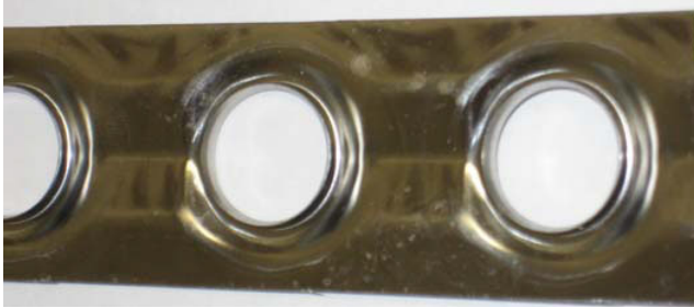
Figure 37: 304 Stainless steel sample before corrosion testing
