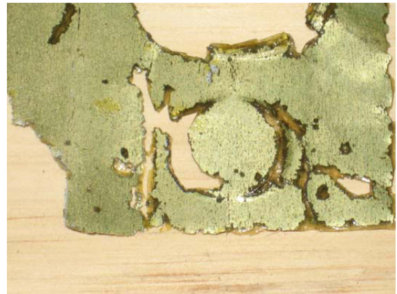
Figure 31: Aluminum polycoat after 250 hours submerged in a 3.9% FRM 63-CB water solution
