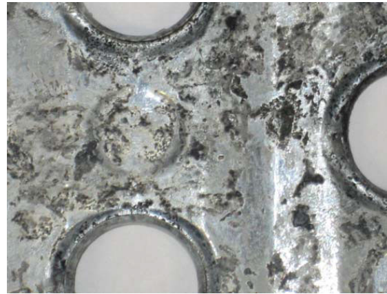
Figure 48: Hot dipped galvanized steel after 250 hours submerged in a .16% Sunny-Sol 150 water solution
