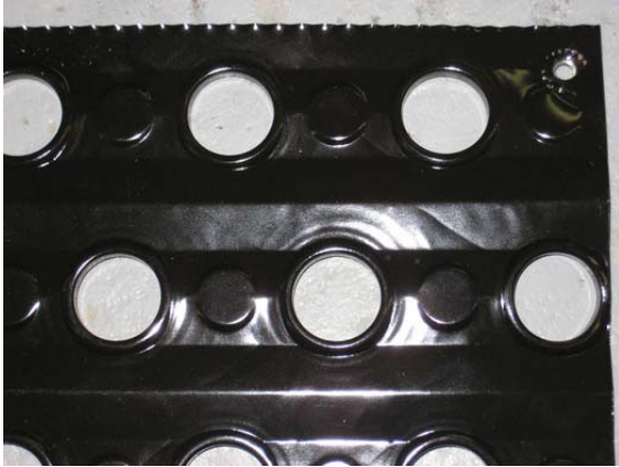
Figure 32: Aluminum Electrofin sample before corrosion testing
