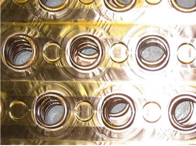
Figure 22: 95/5 Copper-nickel sample before corrosion testing
