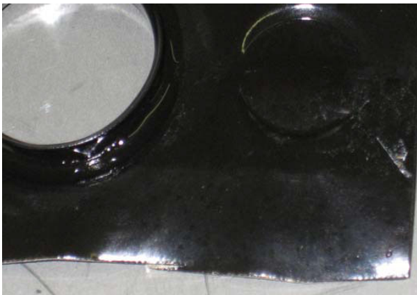
Figure 34: Aluminum Electrofin after 250 hours submerged in a .16% Sunny-Sol 150 water solution
