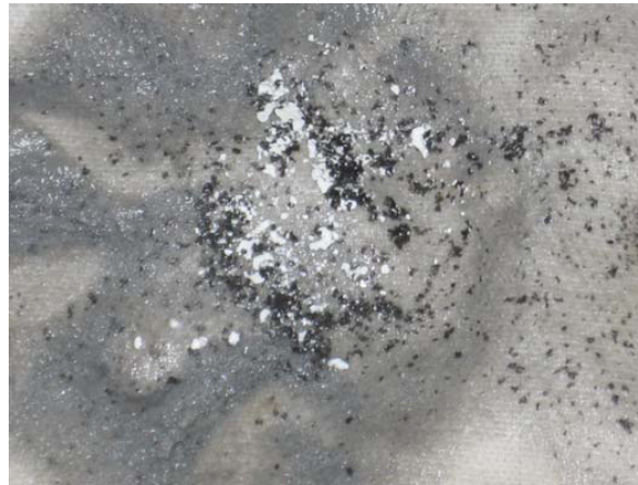
Figure 10: Aluminum 1100 after 250 hours submerged in a 3.9% FRM 63-CB water solution
