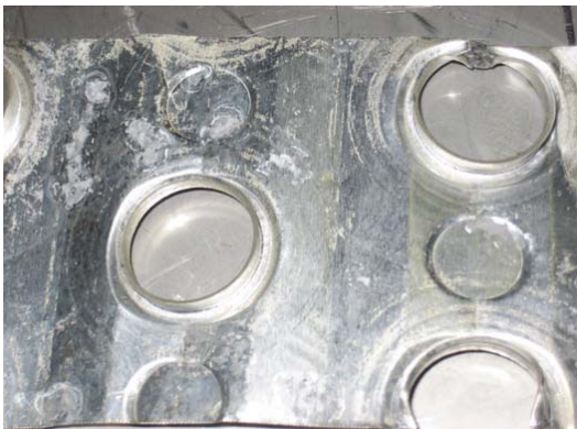
Figure 8: Aluminum 1100 after 250 hours submerged in a .16% Sunny-Sol 150 water solution
