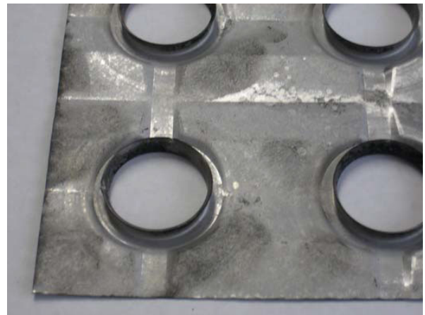
Figure 54: 1100 series aluminum after 500 hours submerged in a 10% ammonium hydroxide solution
