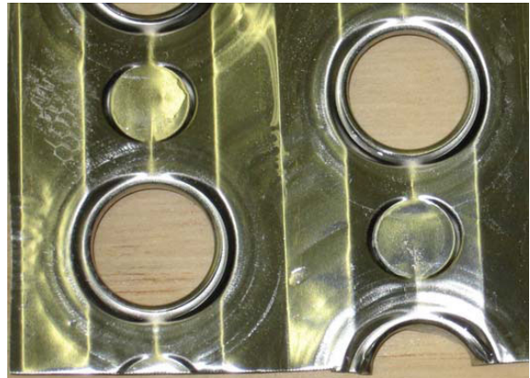
Figure 20: 316 Stainless steel after 250 hours submerged in a 3.9% FRM 63-CB water solution
