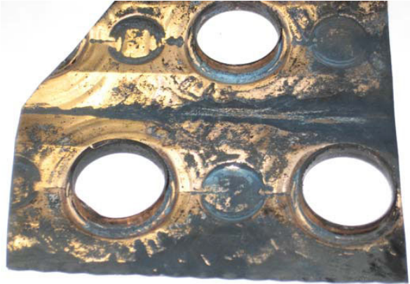
Figure 51: Copper-nickel 95/5 after 500 hours submerged in a 10% ammonium hydroxide solution
