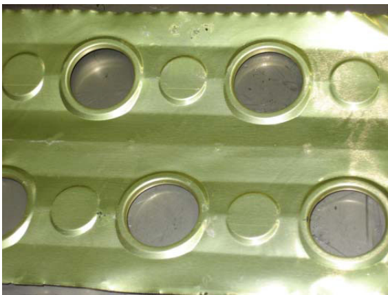
Figure 28: Aluminum polycoat after 250 hours submerged in a .16% Sunny-Sol 150 water solution
