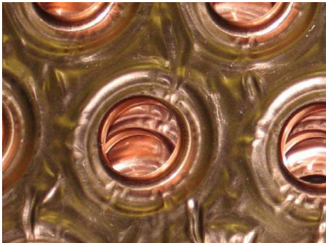
Figure 2: Copper C11000 sample before corrosion testing
