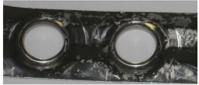
Figure 40: 304 Stainless steel after 250 hours submerged in a 3.9% FRM 63-CB water solution
