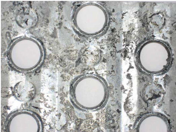
Figure 47: Hot dipped galvanized steel after 250 hours submerged in a .16% Sunny-Sol 150 water solution
