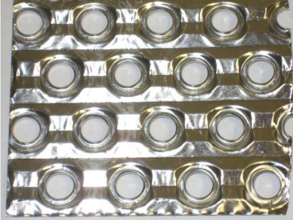
Figure 42: 5052 Aluminum sample before corrosion testing
