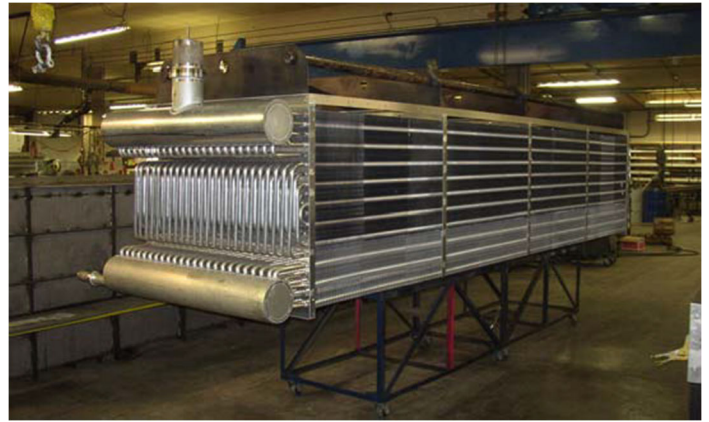
Figure 6 Al/Al Evaporator with Colmac BiM Connections
