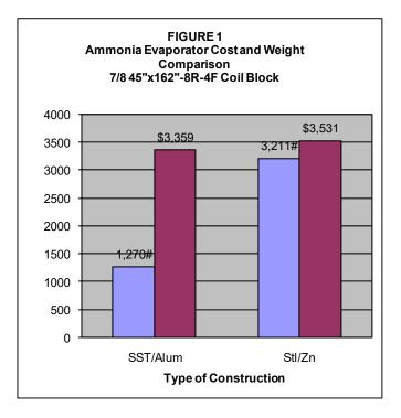
As can be seen in Figure 1, the calculated weight of the galvanized steel (Stl/Zn) coil block (3,211 lbs) is 2 ½ times greater than a stainless tube/aluminum fin (SST/Alum) coil block (only 1,270 lbs) of the same size.
