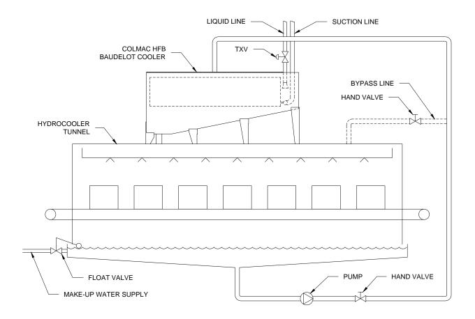
Figure 3 Two-Pump System
