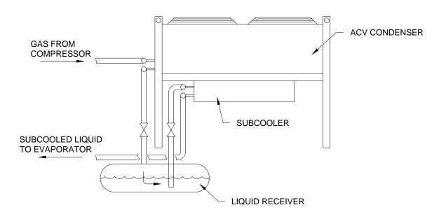
Figure 4 Recommended Subcooler Piping, System with Liquid Pump
