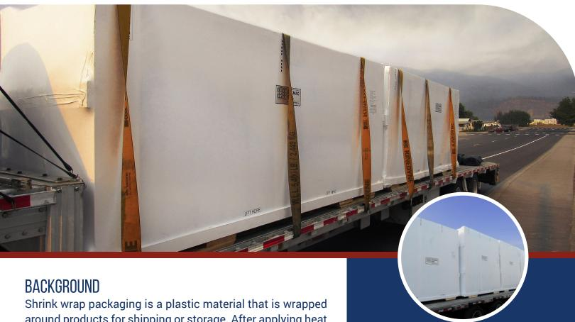
Shrink wrap packaging is a plastic material that is wrapped around products for shipping or storage. After applying heat to the plastic, a tight seal is formed to the exact shape of the product. With a life of 1 to 2 years, products can be stored safely for a significant amount of time.
